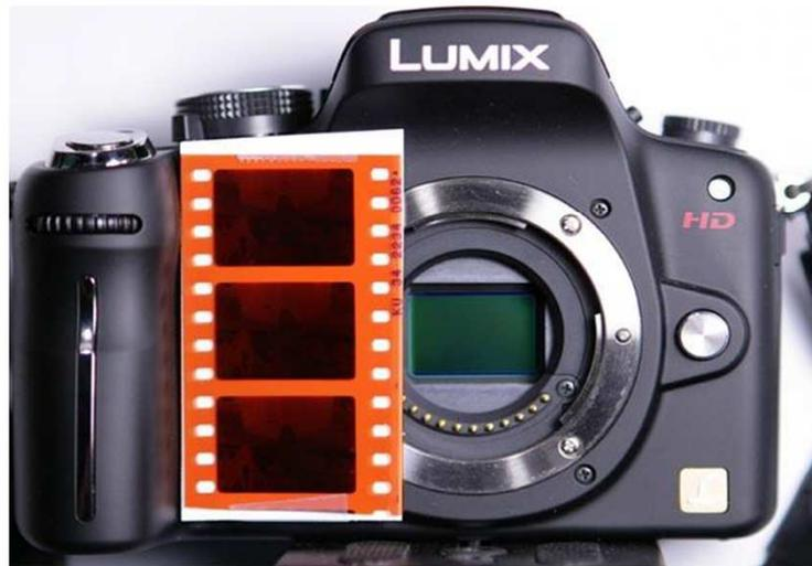
An **image sensor** is a device that converts an optical image into an electronic signal. It is used mostly in digital cameras, camera modules and other imaging devices. Early analog sensors were video camera tubes, most currently used are digital **charge-coupled device (CCD)** or **complementary metal–oxide–semiconductor (CMOS) active pixel sensors**.
