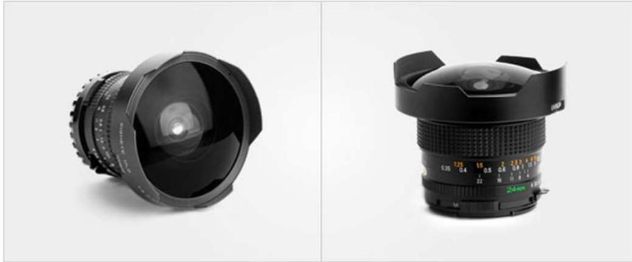
A fisheye lens is a specialized, wide-angle lens that provides extremely wide images by changing straight lines into curves. It can sometimes produce circular, convex, or oval images by distorting the perspective and creating a 180° image. The range of focal length varies between 7~16mm in a fish-eye lens.
